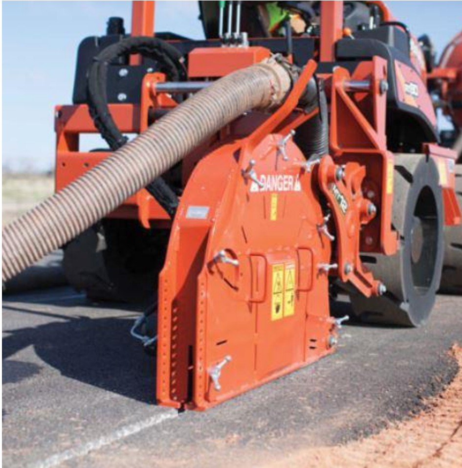
Figure 3 Generic Micro Trenching Machine
