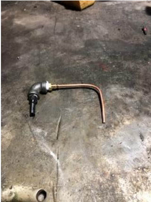
Figure 5 Shop built Pitot Tube using 1/8" Copper Tubing
