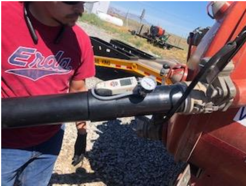
Figure 7 Pitot Tube Flowmeter Assembly installed on a Vac Ex
